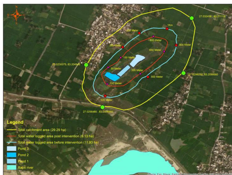
Fig. 2. Spatial analysis of the Mirhiriya wetland system showing catchment extent, interconnected wetlands and reduction in waterlogged area following wetland rejuvenation intervention.
