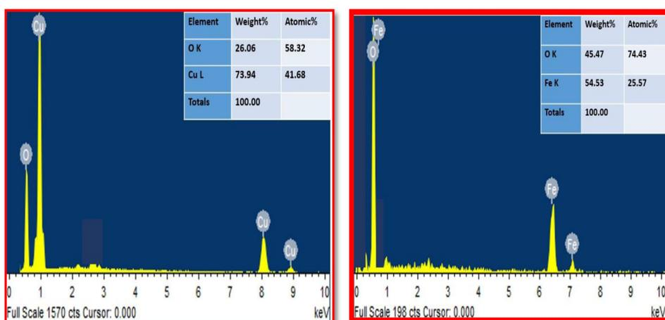
Fig. 3. EDAX Spectra of synthesized copper oxide and iron oxide nanoparticles.
