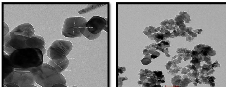
Fig. 4. TEM images of synthesized copper oxide and iron oxide nanoparticles.
