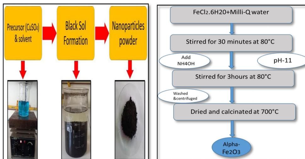
Fig. 1. Synthesis of copper oxide and iron oxide nanoparticles.
