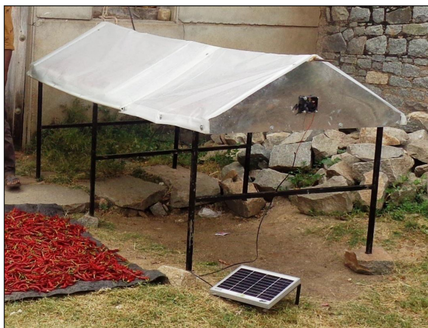
Fig. 2. Convective solar dryer.
