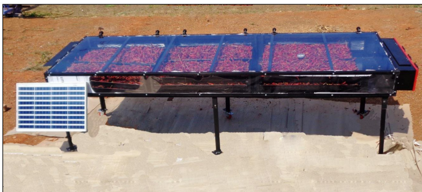
Fig. 1. Box type hybrid energy solar dryer.
