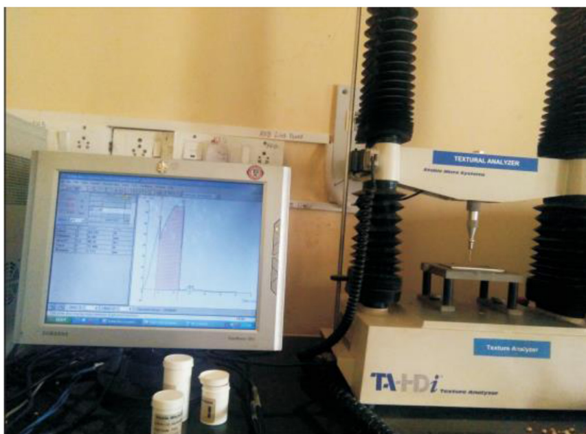
Plate 1. Texture analyzer used for mechanical strength of seed coat (N).
