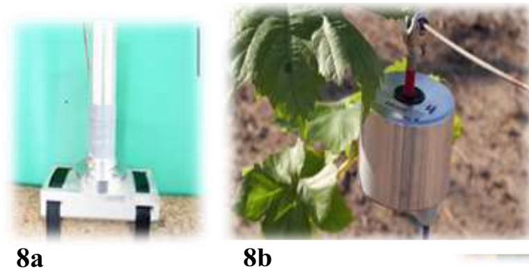
Fig. 8a. Vibration exciter made using Giant magnetostrictive materials. Fig. 8b. Piezo electric Buzzer / Electromagnetic Shaker.
