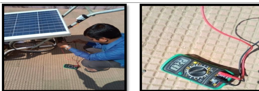
Fig. 9. Testing of battery charging and discharging of solar sprayer with multimeter.
