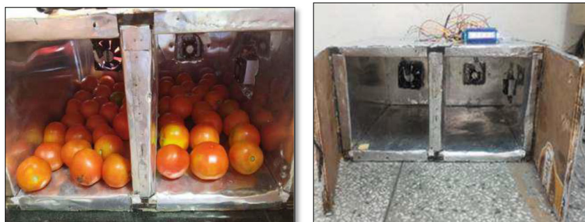
Fig. 2. Multi-cold storage chamber model using Peltier module (with and without load condition).
