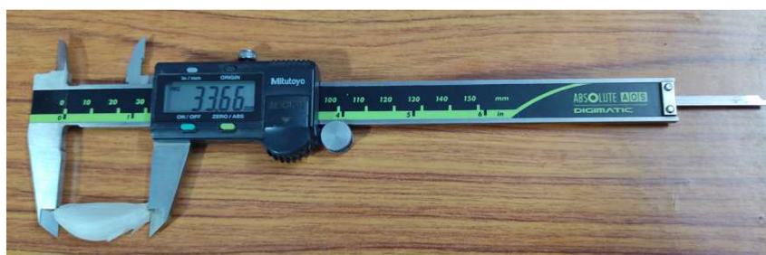
Fig. 1. Measurement of dimensions of garlic clove by using vernier caliper.
