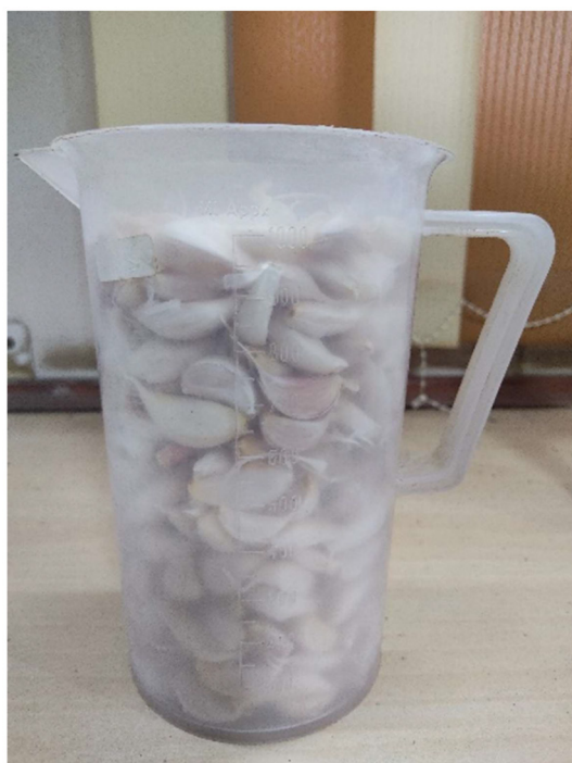
Fig. 2. Determination of bulk density by using measuring cylinder.
