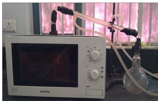
Fig. 1. Microwave assisted essential oil extraction unit.
