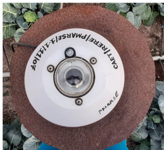
Plate 1. Installation of pyranometer inside the Natural Ventilated Net-cum-Poly house and Shadenet house.
