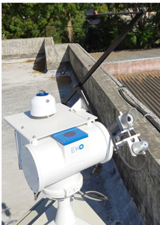
Plate 2. Pyrehelio meter with automatic sun tracking system.
