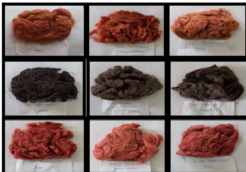
Plate 1. Dyed samples with natural and synthetic mordants using different methods of mordanting.
